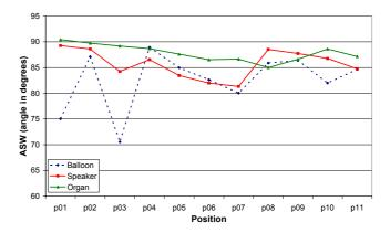
**Figure 4:** Apparent Source Width (ASW) estimation using *IACC<sub>E3</sub>* measurement results.
