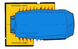
**Figure 1**. Example of coupled volume concert hall: KKL Lucerne, Switzerland (Top & bottom of the map: 4<sup>th</sup> and 3<sup>rd</sup> floors). Blue room: main room with stage and audience; yellow surrounding room: reverberation chamber; red doors: coupling surface. Picture from Beranek [5].
