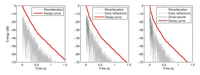
**Figure 7**. Possible refinements of room impulse response synthesis in temporal domain: addition of early reflections (center) and direct sound (right) to reverberation only (left).
