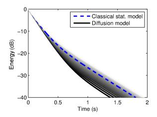
**Figure 4**. Normalized sound energy decays along the line such that Y = 12 m in Fig. 3, i.e. the center line of the main room, for various source-receiver distances 5 < r < 25 m. Darker decays (below) correspond to small r while lighter decays (above) correspond to more distant receivers. The dotted line represents the classical model by Cremer et al. [16].
