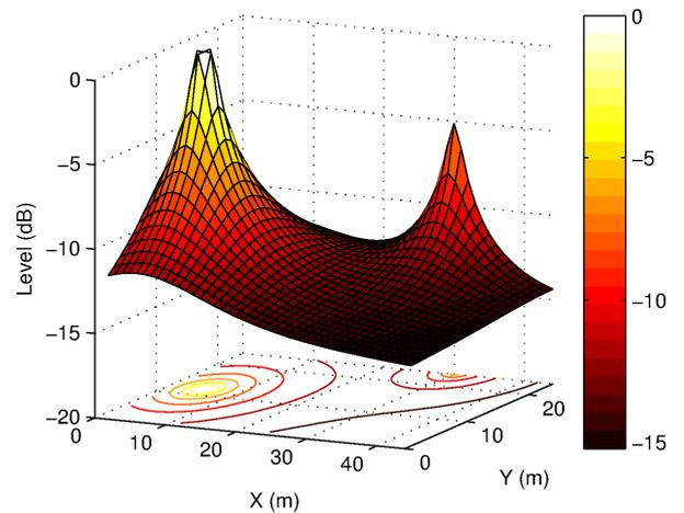
**Figure 3.** Illustration of the output of the model in the case of 2 coupled rooms shown in Fig. 2: sound energy density in the main room. The highest peak corresponds to the sound source on stage, the other one is due to the sound emitted back from the reverberation chamber. Lines on the horizontal plane represent equal energy levels as vertical projections.
