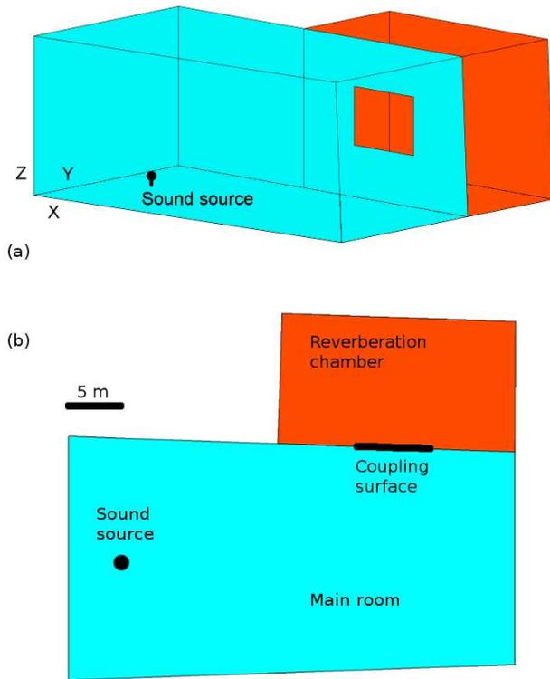
**Figure 2.** (a) View of the coupled room simple geometry used as example. The large blue room on the left is the main room and the orange room behind it is the reverberation chamber. (b) Floor plan of the same geometry.
