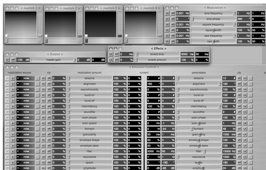
Figure 8. Screen of EmissionControl. The faders on the left determine the amount of modulation of the parameters in the right side. Modulation sources include LFOs and random generators. The joystick controllers at the top let the user manipulate two parameters simultaneously. (The original is in color)
