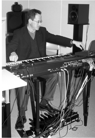
Figure 5. The Creatovox instrument, January 2000. Here I play two simultaneous clouds: one in the bass register (the bass pedal) and one in the high register (keyboard). The left hand manipulates three parameters via a 3D joystick: grain density, grain duration, and amount of reverberation for example, while the right foot controls volume.
