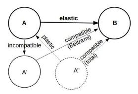
FIGURE 1. The Beltrami decomposition  $(A \to A' \to B)$  vs the standard elastic/plastic decomposition  $(A'' \to A \to B)$
