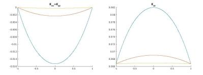
FIGURE 3. Planar (left) and vertical (right) deformations for  $\ell = -10$  (blue),  $\ell = -100$  (red),  $\ell = -1000$  (yellow).
