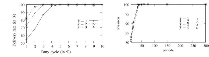
Figure 7. Delivery rate as a function of the duty cycle, for a varying number of possible next hops on a diamond topology.
