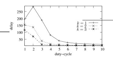
Figure 8. Delay of data frames as a function of the duty cycle, for a varying number of possible next hops on a diamond topology.
