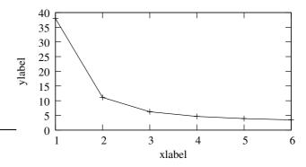
Figure 6. Delay of data frames as a function of the number of next hops, on a diamond topology.
