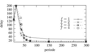
Figure 10. Delay of data frames as a function of the sending period, for three possible next hops on a diamond topology, with a duty cycle of 1%, and for a varying number of fragmentations.
