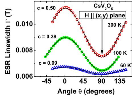
FIG. 8. (Color online) Angular dependence of the ESR linewidth of  $\text{CsV}_2\text{O}_5$  at 300, 100, and 60 K. Symbols represent experimental data points; solid lines are fits to the data using Eq. (3).
