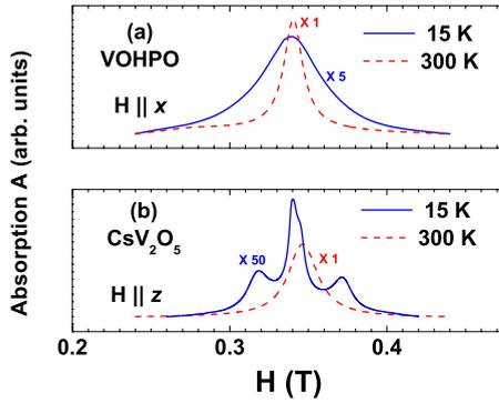
FIG. 4. (Color online) Above: ESR absorption spectra in  $\text{VO}(\text{HPO}_4) \cdot 0.5\text{H}_2\text{O}$  (abbreviated as VOHPO) at 300 K (dashed curve; Lorentzian form) and 15 K (continuous curve; no longer Lorentzian). Below: ESR absorption spectra in  $\text{CsV}_2\text{O}_5$  at 300 K (dashed curve; Lorentzian form) and 15 K (continuous curve; no longer Lorentzian).
