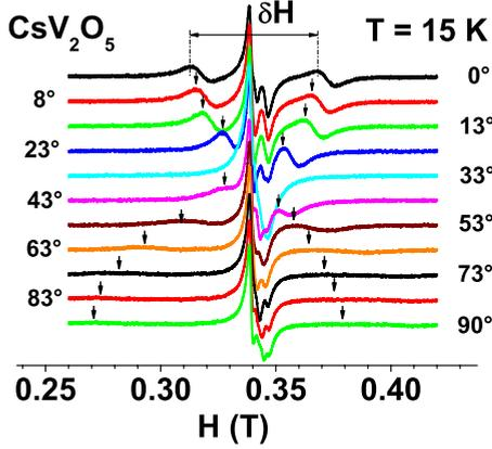
FIG. 9. (Color online) ESR spectra of  $\text{CsV}_2\text{O}_5$  taken at 15 K for different values of  $\theta$  between  $0^\circ$  and  $90^\circ$ . Small arrows indicate the positions of the split-up resonance lines.
