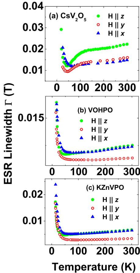
FIG. 7. (Color online) Temperature dependence of the ESR linewidth of (a)  $\text{CsV}_2\text{O}_5$ , (b)  $\text{VO}(\text{HPO}_4) \cdot 0.5\text{H}_2\text{O}$ , and (c)  $\text{KZn}(\text{H}_2\text{O})(\text{VO})_2(\text{PO}_4)_2(\text{H}_2\text{PO}_4)$ , in all three directions,  $x$ ,  $y$ , and  $z$ . The lowest temperature for the plotted data is 19 K in (a) and 14 K in (b) and (c).
