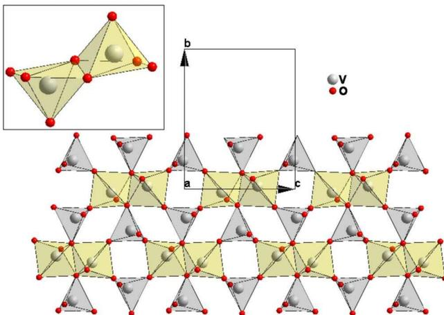
FIG. 3. (Color online) Schematic representation of  $\text{CsV}_2\text{O}_5$  viewed along the  $a$  direction. The basic  $\text{V}_2\text{O}_8$  dimer unit, consisting of two edge-sharing  $\text{VO}_5$  square pyramids, is sketched at the top left corner of the figure.
