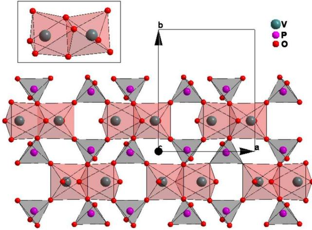
FIG. 2. (Color online) Schematic representation of the structure of  $\text{KZn}(\text{H}_2\text{O})(\text{VO})_2(\text{PO}_4)_2(\text{H}_2\text{PO}_4)$  viewed along the  $c$  direction. The basic  $\text{V}_2\text{O}_9$  dimer unit, consisting of two  $\text{VO}_6$  octahedra sharing one face, is sketched at the top left corner of the figure.
