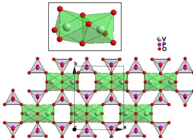
FIG. 1. (Color online) Schematic representation of  $\text{VO}(\text{HPO}_4) \cdot 0.5\text{H}_2\text{O}$  in the  $(a, b)$  plane. The basic  $\text{V}_2\text{O}_9$  dimer unit, consisting of two  $\text{VO}_6$  octahedra sharing one face, is sketched at the top of the figure.
