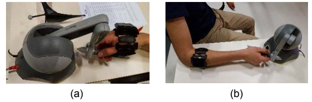
Figure 4: Locations of both force and vibrotactile cues: (a) Co-located; and (b) Dislocated.
