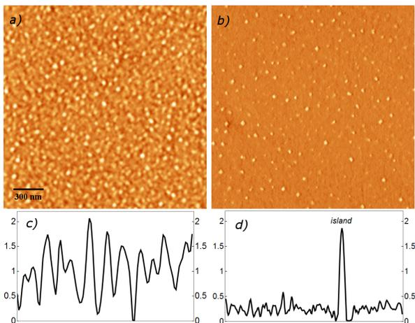
Figure 2: AFM images of (a) 2nm  $\text{Si}_{0.5}\text{Ge}_{0.5}$  and (b) 1.3nm  $\text{Si}_{0.4}\text{Ge}_{0.6}$  films deposited on Si(001). The image sizes are  $2\mu\text{m}\times 2\mu\text{m}$  and their vertical scale is 7 nm. Images (c) and (d) are lines profiles corresponding respectively to (a) and (b).
