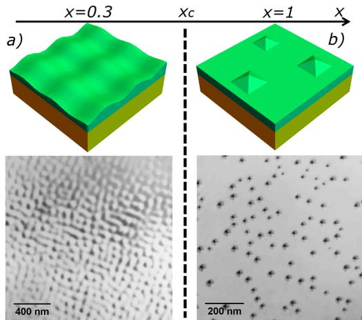
Figure 1: Graphical representation and TEM plane view images of the two growth modes at work in SiGe strained films ; a) at low strain for a typical  $\text{Si}_{0.7}\text{Ge}_{0.3}$  film on Si(001) and b) at high strain for a typical Ge film on Si(001).
