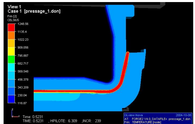
Fig. 13. Temperature distribution in gob and moulds at the end of pressing
