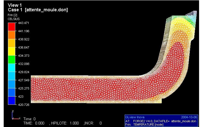
Fig. 8. Initial condition of the mould for the loading stage
