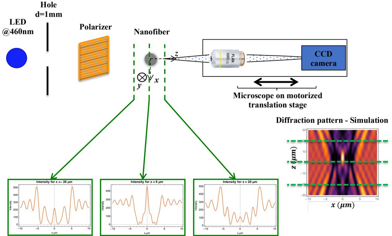
Fig. 1. The microscope with its illuminating system
