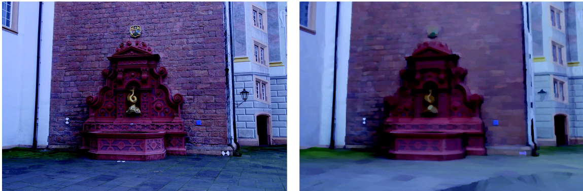
Fig. 8. Left: One real view of the object ‘fountain-P11’ [13]. Right: Colored estimated albedo, using the proposed approach. Geometry and camera parameters estimates are outputs of an SfM/MVS pipeline using 25 input images. Only 8 images have been used as inputs of our algorithm. (Color figure online)
