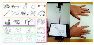
Figure 1. Diagrams used (left) and experimental setup (right): a raised-line drawing is placed over the touchscreen. A camera located above the drawing tracks fingers movements.
