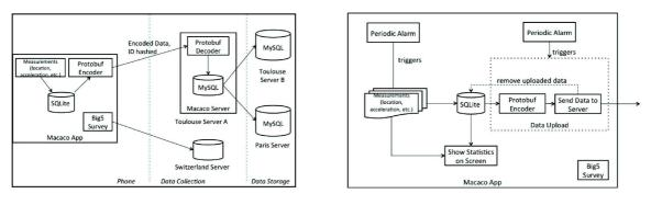
Fig. 1. Overall Macaco crowdsensing architecture (left) and Macaco app architecture (right)
