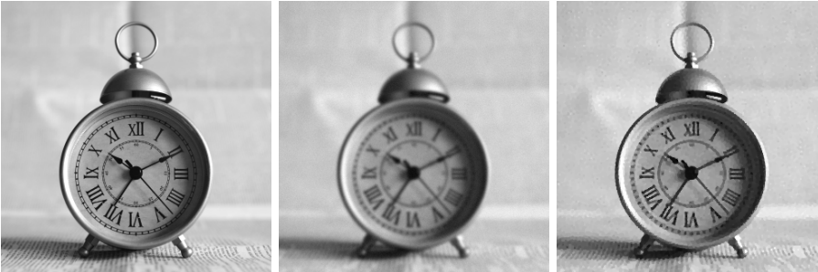
FIG. 14. Left: original “clock” image, middle: with a Gaussian blur of std. dev. 1.5 and a 1% Gaussian noise, right: TV-regularised deblurred image with (B.2).
