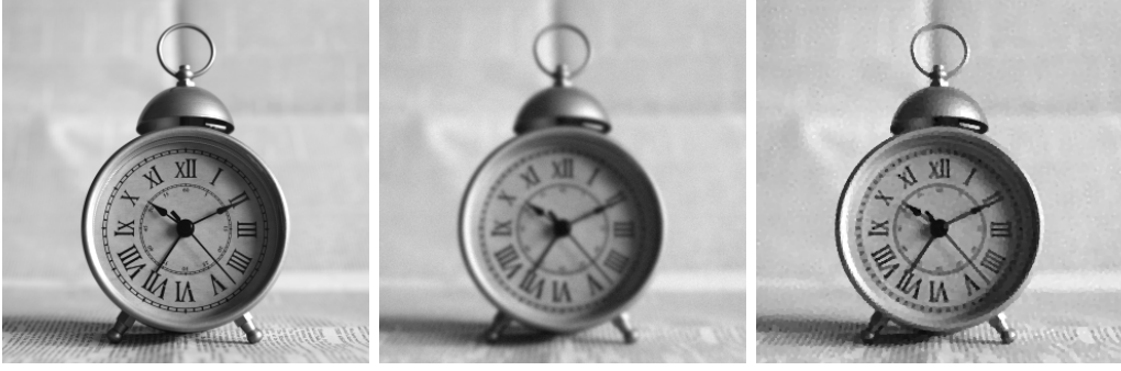
Figure 14: Left: original “clock” image, middle: with a Gaussian blur of std. dev. 1.5 and a 1% Gaussian noise, right: TV-regularised deblurred image with (49).
