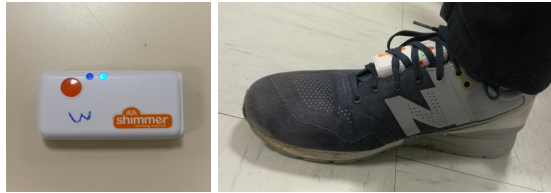
Figure 3: Shimmer3 sensor and placement on the shoe.
