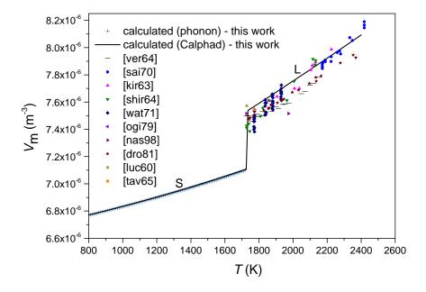
Figure 6: Calculated Ni molar volume increase at the melting point. Experimental data from Vertman  $et\ al.,^{24}$  Tavadze, <sup>33</sup> Saito and Sakuma, <sup>25</sup> Kirschenbaum and Cahill, <sup>26</sup> Shiraishi and Ward, <sup>27</sup> Watanabe  $et\ al.,^{28}$  Ogino  $et\ al.,^{29}$  Nasch and Manghnani <sup>30</sup> and Drotning. <sup>31</sup>
