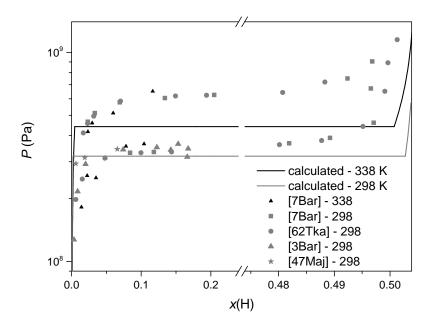
Figure 12: Pressure-composition isotherms at 298 and 338 K. Experimental measurements of Baranowski,  $^{63,64}$  Tkacz  $^{65}$  and Majchrzak.  $^{62}$
