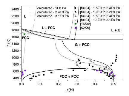
Figure 14: Ni–H phase diagrams at several pressures highlighting the miscibility gap formation. Experimental solubility branches of the miscibility gap of Antonov  $et~al.^{69}$  and Fukai  $et~al.^{56}$  solubility data in the hydrogen rich fcc phase  $^{56}$  measured on a hydrogenated sample during cooling (empty symbols) or heating (filled symbols) and 3-phase equilibrium of Serdyuk  $et~al.^{70}$
