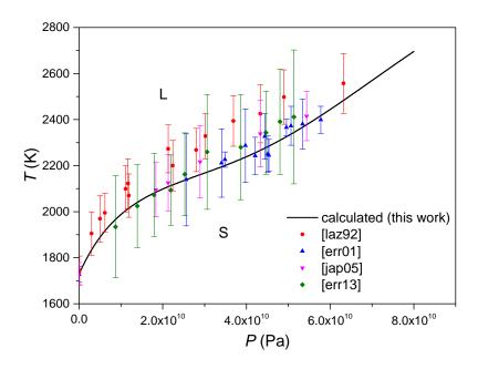
Figure 5: Calculated P-T phase diagram of pure Ni. Experimental data from Lazor  $et\ al.$ ,  $^{36}$  Errandonea  $et\ al.$ ,  $^{37}$  Japel  $et\ al.$  and Errandonea.  $^{39}$
