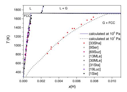
Figure 9: Calculated Ni–H phase diagrams at moderate pressure:  $1.0\times10^5\,\mathrm{Pa}$  (blue solid line) and  $1.0\times10^7\,\mathrm{Pa}$  (black dashed line). Experimental isobaric measurements of Sieverts,  $^{40}$  Shapovalov and Serdyuk,  $^{41}$  Serdyuk and Chuprina,  $^{42}$  Suzuki and McLellan,  $^{43}$  Mc Lellan and Sutter,  $^{44}$  McLellan and Oates,  $^{74}$  Stafford and McLellan  $^{45}$  and Luckemeyer-Hasse and Schenck.  $^{46}$
