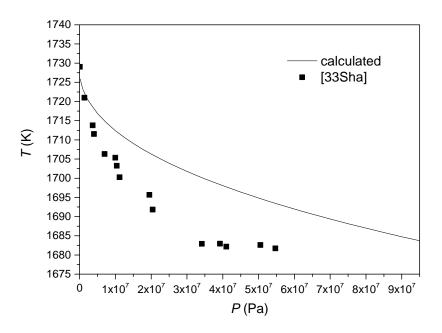
Figure 10: Solid-liquid-gas equilibrium temperature as a function of pressure compared with the data of Shapovalov and Serdyuk.<sup>41</sup>
