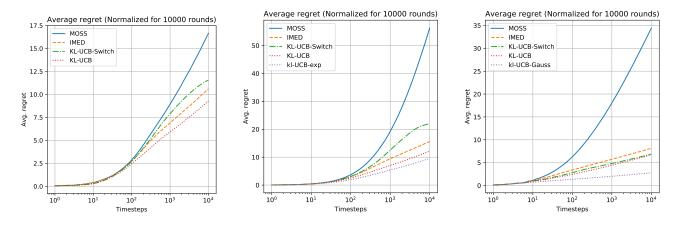
Figure 1: Regrets approximated over 10,000 runs, shown on a logarithmic scale; distributions of the arms consist of: Left: Bernoulli distributions with parameters (0.9, 0.8)
