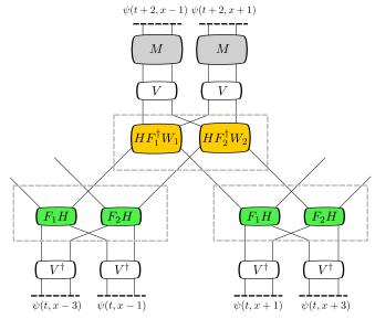
FIG. 5: (1+1) implementation with U(2) gates. Here  $M=e^{2\varepsilon \mathrm{i}C}$  implements the mass.
