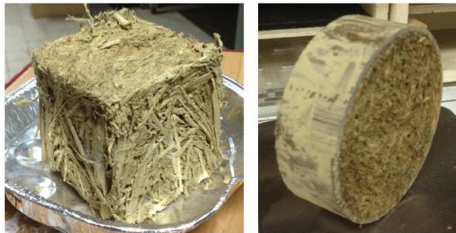
Fig. 1: Straw clay samples with different geometries
