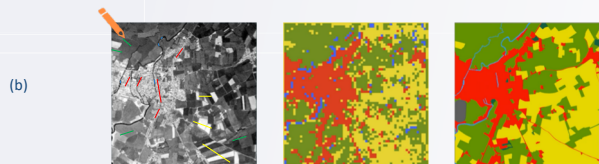
Fig. 3 : (a) Software workflow, (b) Left - scribbled historical aerial image ; Center - result with the software learning solely from scribbles ; Right - ground truth, unseen by the software
