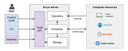
Fig. 1. Overview of ACCIO's architecture: users use a client application to interact with the server, which in turn interacts with a library of ACCIO operators deployed on some computing resources.
