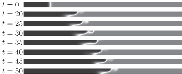
FIG. 7. Periodic time evolution of the concentration field in the presence of antagonistic solutal and thermal Marangoni effects when the front remains unsteady in the co-moving frame: Ma_c = -70 and Ma_T = 200 . The other parameters are Le = 10 and L_z = 10 .
