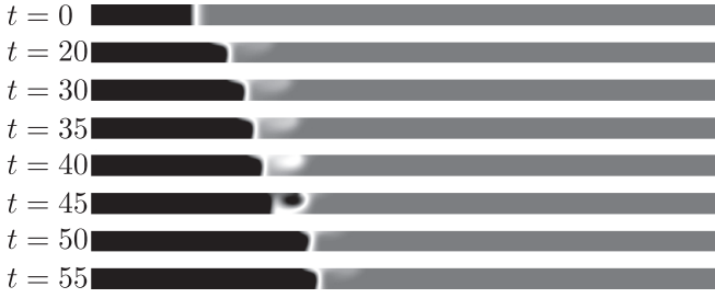
FIG. 4. Periodic time evolution of the concentration field in the presence of antagonistic solutal and thermal Marangoni effects when the front remains unsteady in the co-moving frame: Ma_c = -80 and Ma_T = 100 . The other parameters are Le = 10 and L_z = 10 .
