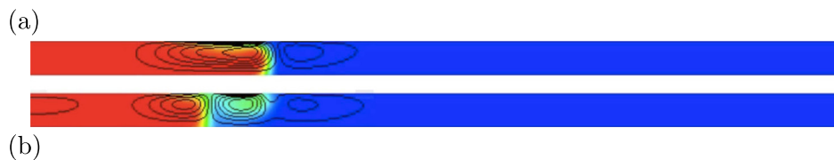
FIG. 5. Streamlines superimposed on the concentration field in the presence of antagonistic solutal and thermal Marangoni effects for Ma_T = 100 , Le = 10 , L_z = 10 , t = 40 for (a) a steady case, Ma_c = -180 , and (b) an unsteady case, Ma_c = -80 . The concentration ranges here from c = 1 (products to the left) shown in red to c = 0 (reactants to the right) shown in blue. The streamlines correspond to iso-contours of the streamfunction, \psi , equally spaced between the maximum value of \psi and 0.
