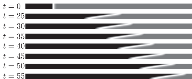
FIG. 2. Time evolution of the concentration field in the presence of cooperative solutal and thermal Marangoni effects: Ma_c = 20 and Ma_T = 100 . The other parameters are Le = 10 and L_z = 10 .
