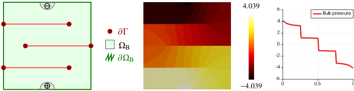
(a) Domain configuration (left), bulk pressure p (middle) and bulk pressure profile over x_1 = 0.5 (right).
