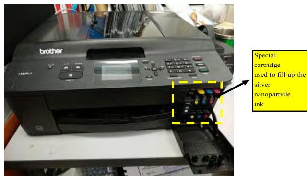
FIGURE 9. Brother MFC-J430W printer with special cartridge filled with silver nanoparticles ink used for fabricate the FSS prototype.
