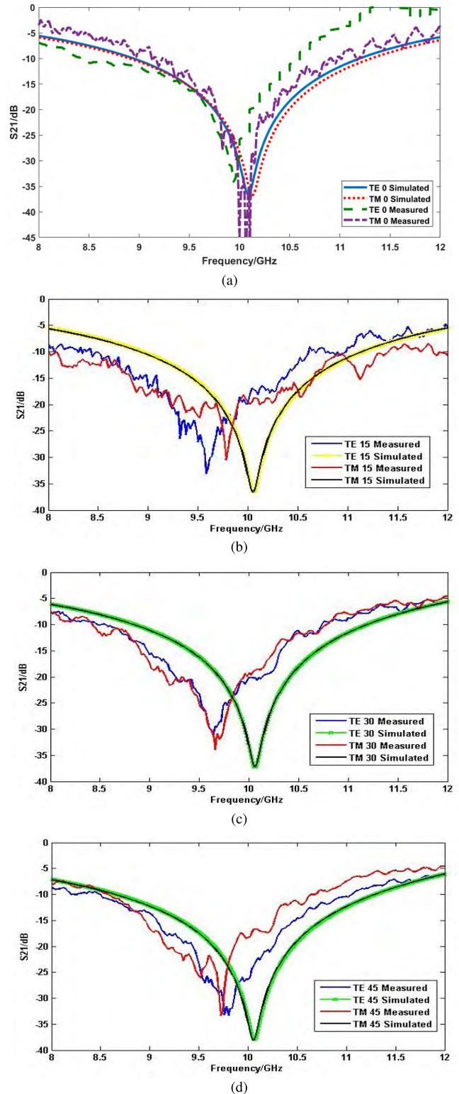
**FIGURE 11.** Comparison of the simulated and measured transmission response for TE and TM polarization at (a)  $\theta = 0^\circ$ , (b)  $\theta = 15^\circ$ , (c)  $\theta = 30^\circ$  and (d)  $\theta = 45^\circ$ .
