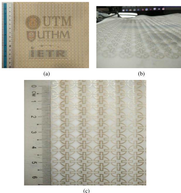
FIGURE 15. Fabricated row-by-row unit cell FSS prototype (a) top view, (b) side view, and (c) zoom view.
