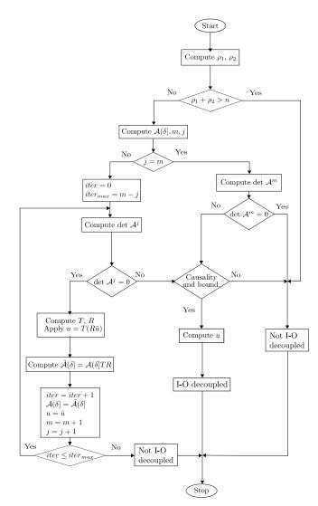
Fig. 1. Input-output decoupling algorithm
