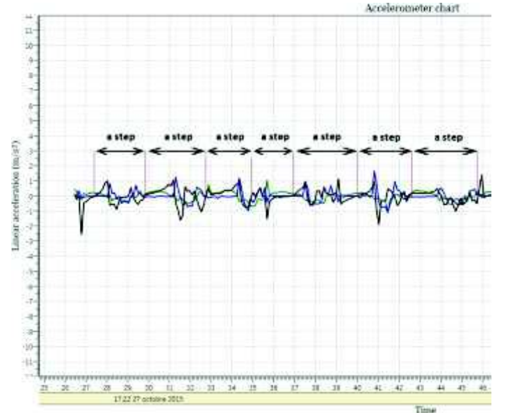
Fig. 6. Detection of a step through the linear acceleration.
