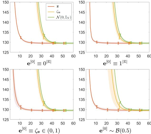
Figure 4: Performances of SL-PAM with different initial values of  $\mathbf{u}^{[0]}$  and  $\mathbf{e}^{[0]}$ , when the input is the image in Fig. 2, degraded by additive white Gaussian noise with standard deviation  $\alpha = 0.04$ . SL-PAM is not sensitive to the initialization.
