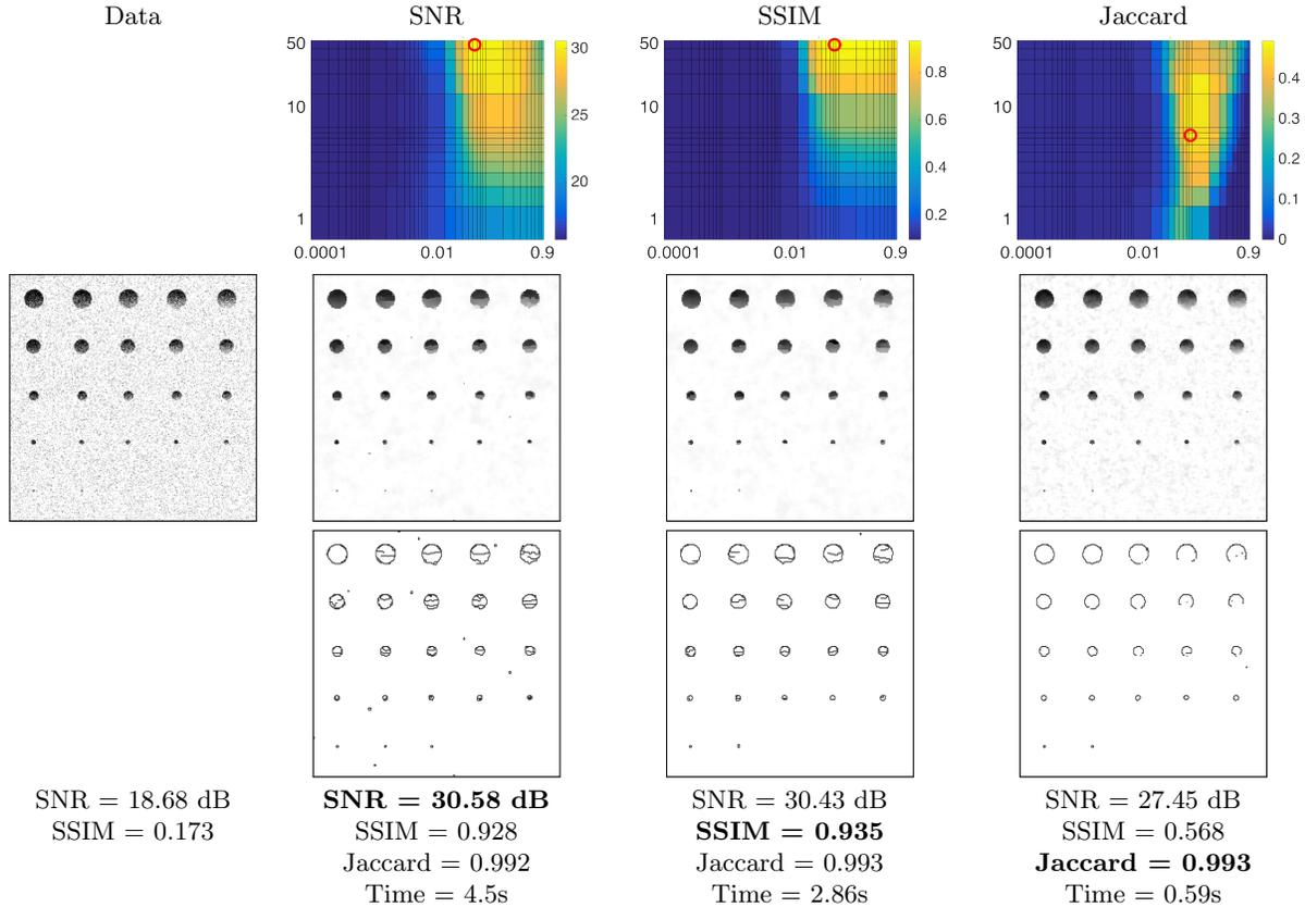
Figure 7: Denoising with SL-PAM and the quadratic- $\ell_1$  penalization on the image in Fig. 2, degraded by additive white Gaussian noise with standard deviation  $\alpha = 0.16$ . The best results for each score are presented.
