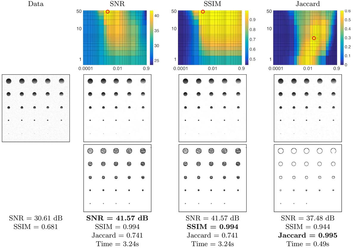
Figure 6: Denoising with SL-PAM and the quadratic- $\ell_1$  penalization on the image in Fig. 2, degraded by additive white Gaussian noise with standard deviation  $\alpha = 0.04$ . The best results for each score are presented.
