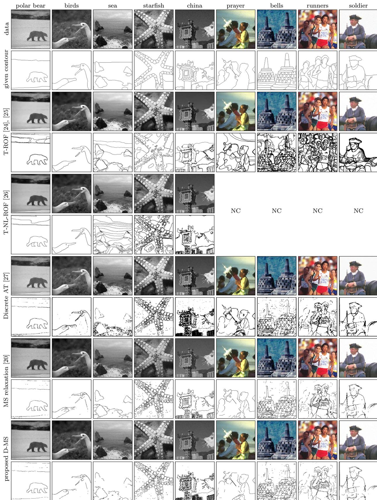
Figure 8: Comparison according to the SNR and the Jaccard of denoising and contour detection performances, involving white Gaussian noise with standard deviation  $\alpha = 0.05$ , with state-of-the-art methods, from top to bottom: T-ROF [23, 24], T-NL-ROF [28], the Discrete AT [29], the MS relaxation [27], and the proposed method (D-MS).
