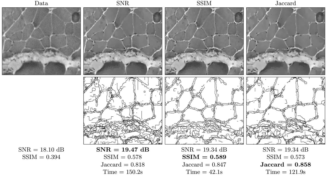
Figure 13: Image restoration with with SL-PAM and the quadratic- $\ell_1$  penalization on the image in Fig. 2 degraded by additive white Gaussian noise with standard deviation  $\alpha = 0.2$  and a Gaussian blurring filter of size  $7 \times 7$  and standard deviation  $\sigma = 2$ . The best results for each score are presented.
