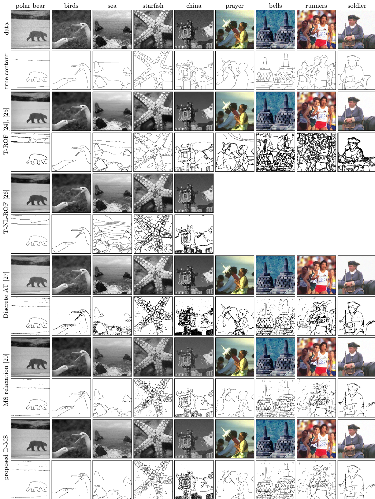
Figure 8: Comparison according to the SNR and the Jaccard of denoising and contour detection performances, involving white Gaussian noise with standard deviation \alpha = 0.05 , with state-of-the-art methods, from top to bottom: T-ROF [24, 25], T-NL-ROF [26], the Discrete AT [27], the MS relaxation [20], and the proposed method (D-MS).
