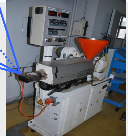
Single screw extruder φ 30 mm, L/D 24 mm
