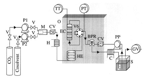
V: 2 way valves; P1, P2: high pressure pumps; M: mixer; CV: checking valve; H: heater;
