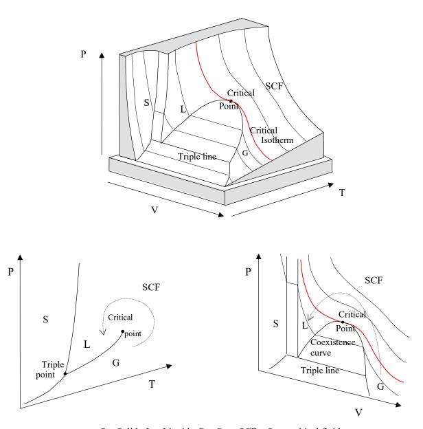
S = Solid; L = Liquid; G = Gas; SCF = Supercritical fluid
