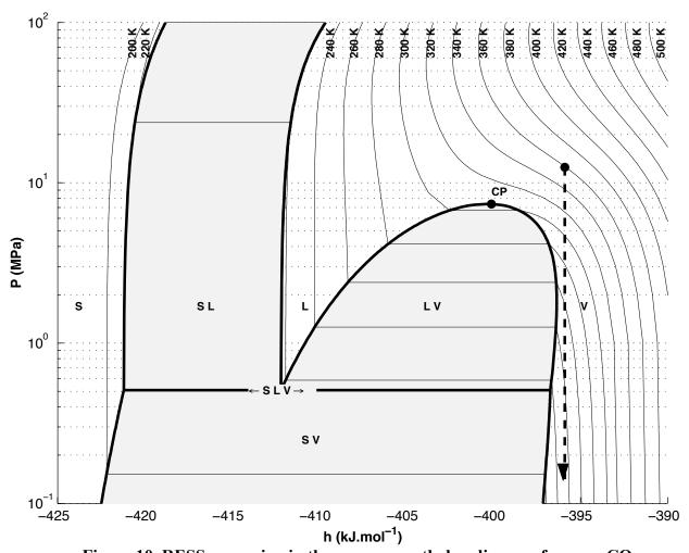
Figure 10. RESS expansion in the pressure-enthalpy diagram for pure CO<sub>2</sub>
