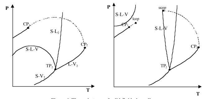
Figure 6. The main types of solid-fluid phase diagrams
