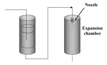
Figure 15. The PGSS process: schematic flow diagram
