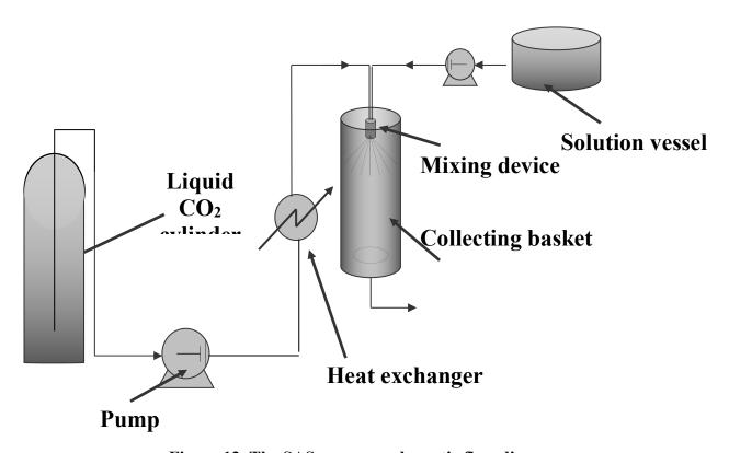
Figure 12. The SAS process: schematic flow diagram
