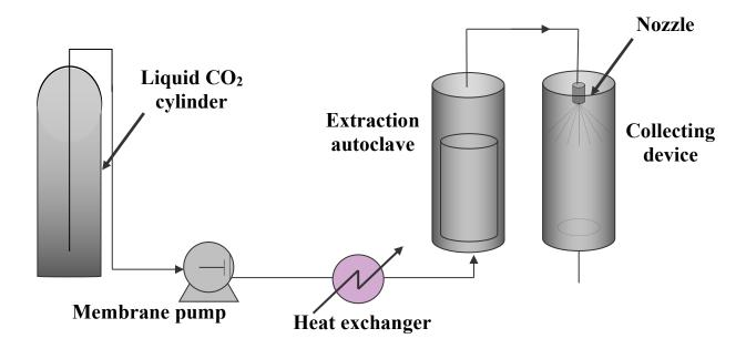
Figure 9. The RESS process: schematic flow diagram
