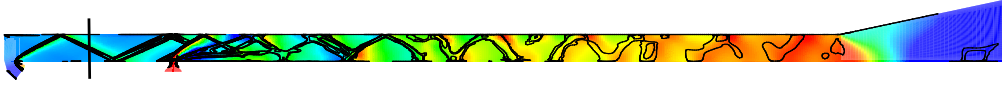
FIGURE 1. Slice through the injector from a RANS simulation at the nominal operating condition. Contours of pressure showing the gradual increase caused by combustion, overlaid with contour lines of large negative dilation showing the strongest shocks. The vertical line before the injector shows the location of the inflow for the LES.
