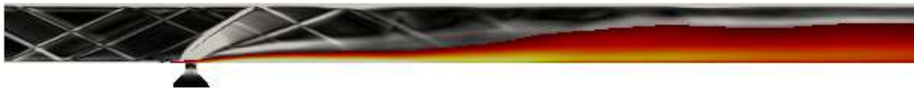
FIGURE 10. Composite simulated Schlieren |\nabla\rho| in a slice through the injector and line-of-sight integrated mean \text{OH}^* chemiluminescence in the first half of the combustion chamber.
