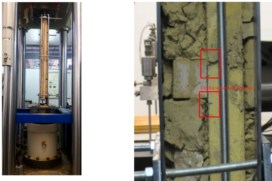
Figure 8. Experimental setup (left) and displacement at the interface between shear band and mortar layer (right)
