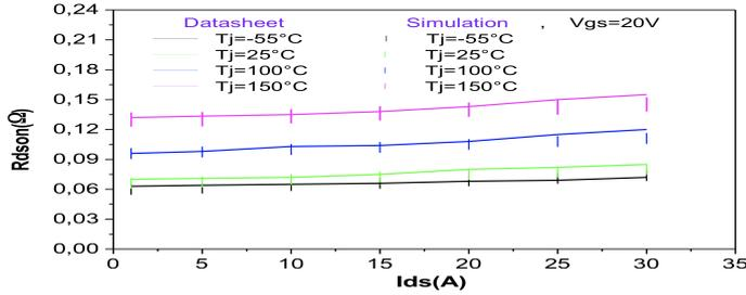
Fig. 9.  $R_{DSon}$  Variations in function of the junction temperature
