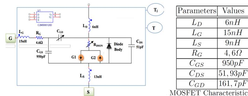
Fig. 7. Pspice Sic MOSFET C2M0080120D and Parameters
