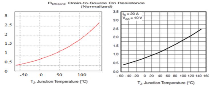
**Fig. 11.** Variation of  $R_{DSon}$  versus the temperature  $T_j$
