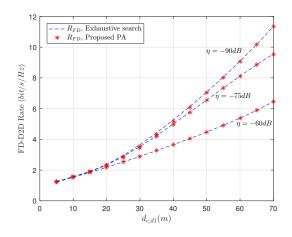
Fig. 5. Comparison of FD-D2D rate obtained from the exhaustive search and from our proposed power allocation scheme in the asymmetric case
