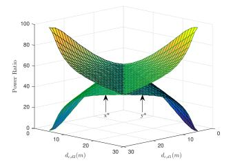
Fig. 6. The optimal power ratios variation w.r.t to CUE location. $(\eta = -70 dB)$
