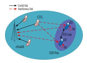
Fig. 1. A FD-D2D pair shares the resources of one cellular user, which creates interference between the two types of links.
