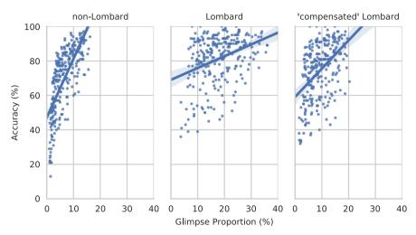
Fig. 6. Accuracy versus GP for different Lombard conditions. Each point represents the averages of an individual speaker at a particular SNR. The line represents the linear regression to the data points and the shaded area around the line the 95% confidence interval for the regression estimate.
