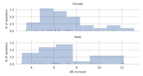
Fig. 3. Distribution of per-speaker average energy gains in dB between non-Lombard and Lombard speech. Each dark tick on the x-axis represents the average energy gain of an individual speaker.
