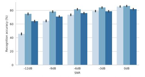
Fig. 4. Recognition accuracies for different SNR values and testing speech conditions. All models have been trained on matched conditions. From light to dark: non-Lombard, Lombard, 'compensated' Lombard. The height indicates the average across utterances while the black line depicts the standard error.
