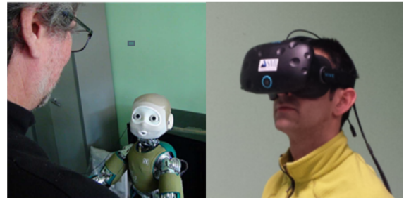
Figure 1 Our humanoid robot Nina remotely controlled via our teleoperation/being platform.
