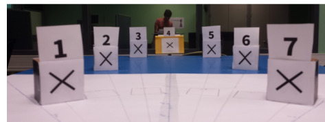
Figure 6 Arrangement of the 7 physical targets used in the validation experiment. We mainly vary the target depths. Pilots are asked to fixate the crosses on the cubes whose target numbers that are instructed verbally.
