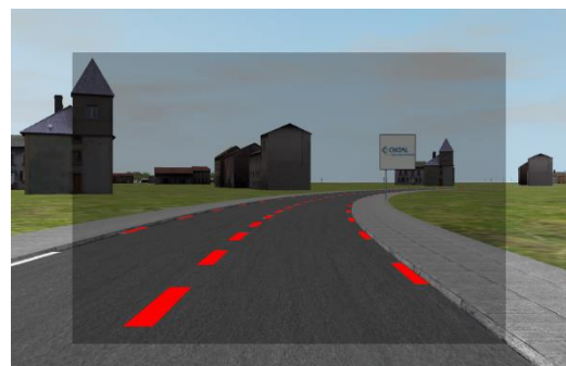
Figure 1. Designed AR-HUD "Lane marking highlight"
