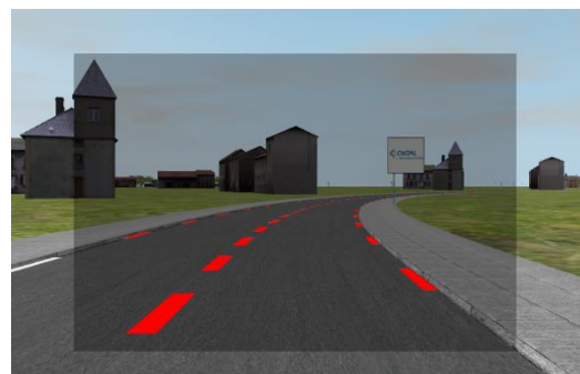
Figure 1. Designed AR-HUD "Lane marking highlight"
