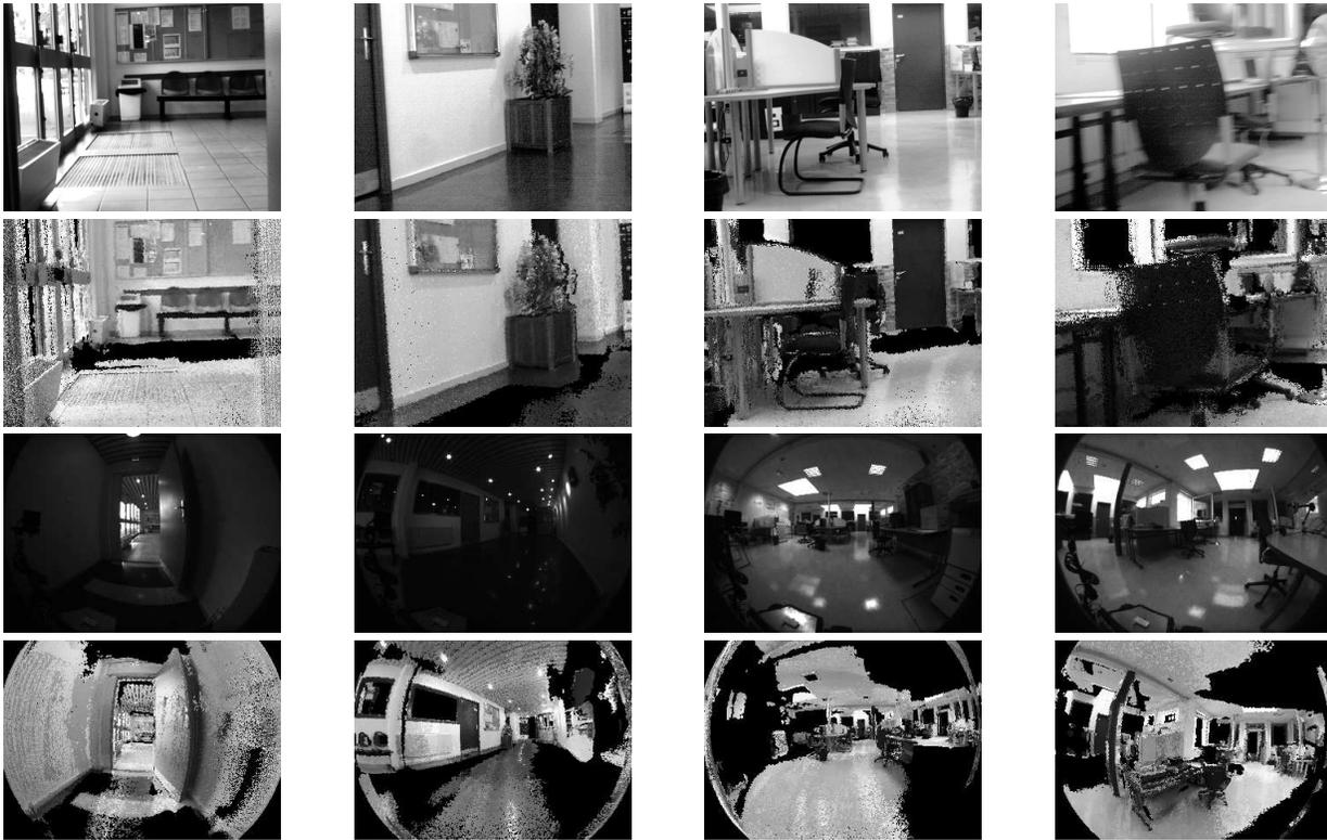
Fig. 5: Near-infrared and polarization images given in inputs of the registration method (first and third rows), virtual images rendered at the virtual camera poses estimated using the proposed registration method (second and fourth rows)
