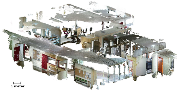
Fig. 3: A 3D model of an indoor building environment created from Kinect data acquired by the Summit XL robot
