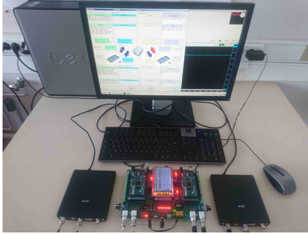
Figure 5: The platform involving the sensors, the touch screen, the Arduino MEGA cards and the oscilloscopes to visualize the analog signals.
