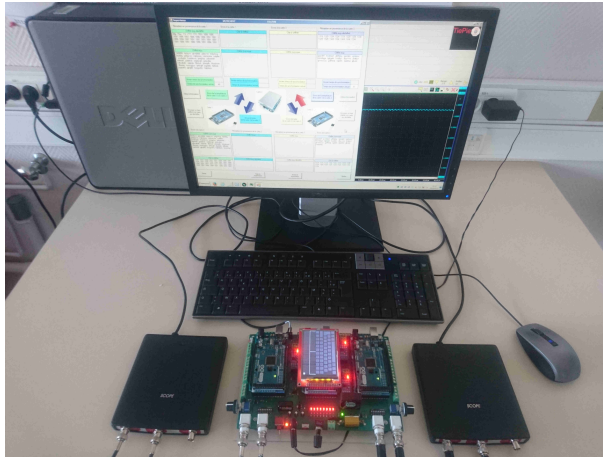
Figure 5: The platform involving the sensors, the touch screen, the Arduino MEGA cards and the oscilloscopes to visualize the analog signals.
