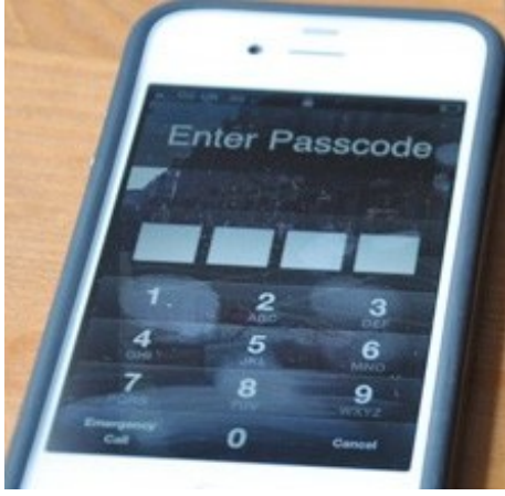
Fig. 7: Example of a smudge attack.
