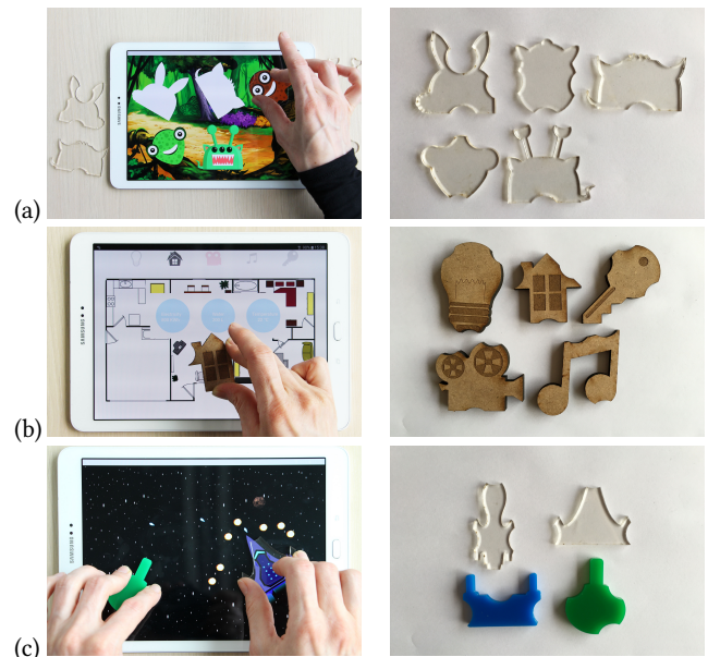
Figure 6: The three proof-of-concept token sets: (a) toy characters, (b) home automation, (c) spaceship game.
