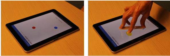
Figure 3: A trial to collect comfortable tripod grasps. (Left) Two circles indicate where to put the physical ruler (red circle: middle, blue circle: thumb). (Right) Participants slide their index to turn yellow the area within which this latter finger can be without making the hand posture become uncomfortable.
