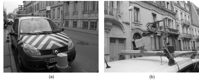
Figure 6. Illustration of a car parked in the street with the radiometer on the front bumper (a), and details of instruments installed on the vehicle roof.
