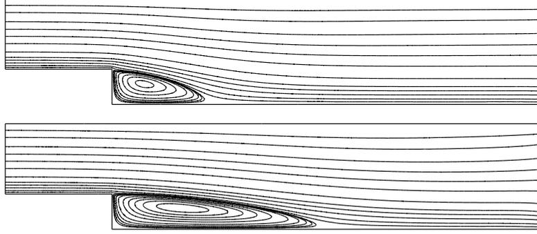
FIGURE 6. Streamlines of the steady state solution at  $\nu = 1/50$  (top) and  $\nu = 1/150$  (bottom);  $L = 15$ .
