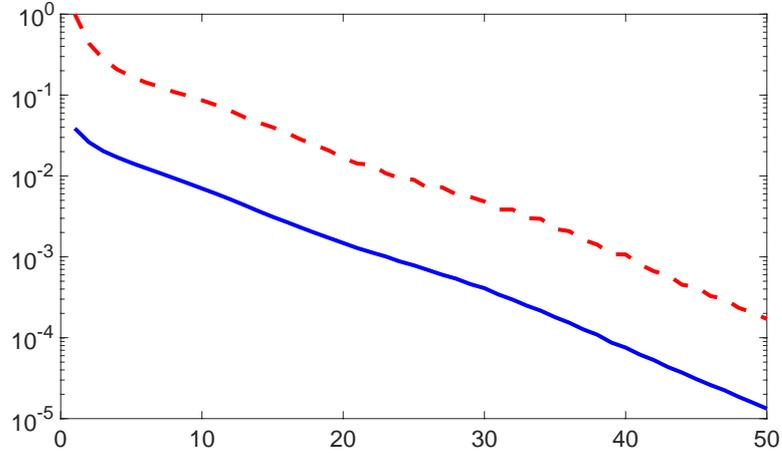
FIGURE 3. Evolution of  $\sqrt{E(\mathbf{y}^k)}$  (blue full line) and the norm  $\|\mathbf{g}^k\|_{\mathbf{H}^1}/\|\mathbf{g}^0\|_{\mathbf{H}^1}$  (red dashed line) w.r.t. iterate  $k$  of the CG algorithm -  $\nu = 1/50$ .
