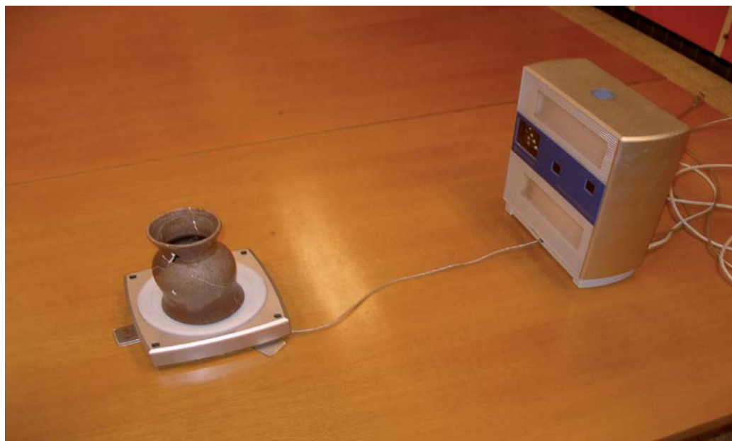
Fig. 12. Scanner de table NextEngine.
